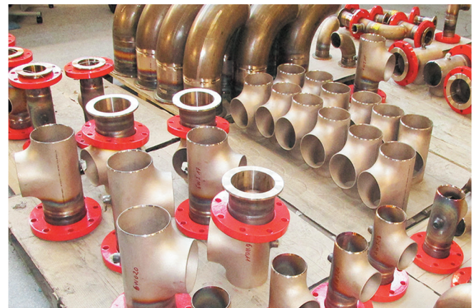
90/10 CuNi piping spools
