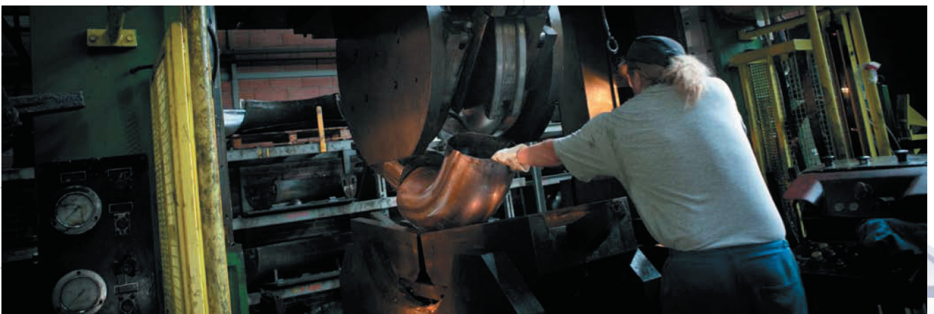
Cold forming CuNi elbows from seamless pipes
