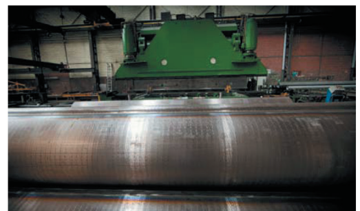
U-BEND PRESS CuNi pipe forming
