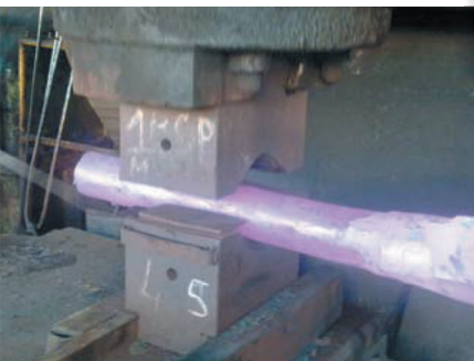
Hot forging of CuNi bar
