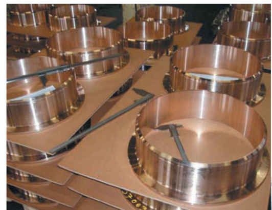
CuNi Inner flanges final inspection
