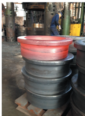
Hot forging of 20" CuNi stub ends
