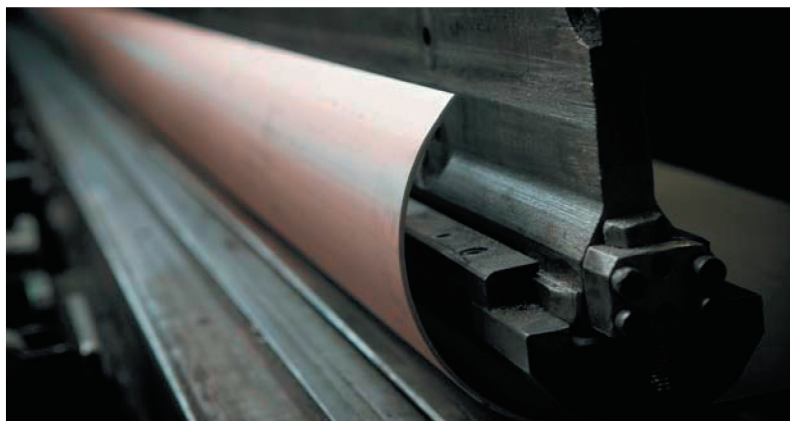
U-BEND PRESS forming CuNi plate into pipe
