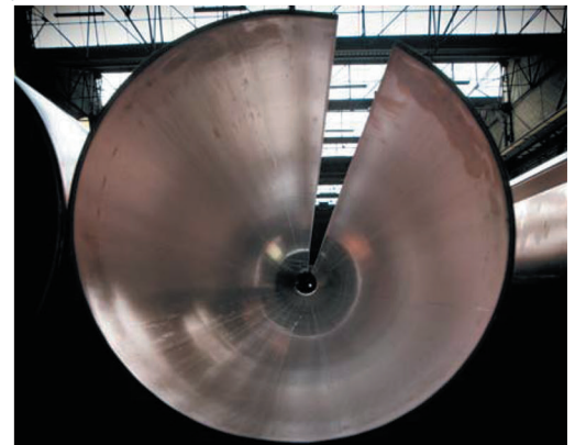
3 ROLLS CuNi pipe forming
