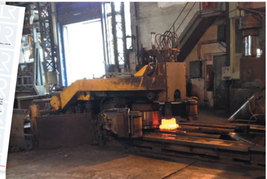
Hot ring rolling of CuNi flange
